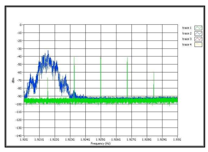
Note 1: The interference of level on f2 is TL+UM+1dB. The interference of level on f1 is TL+UM-6dB. The level of other 3 carriers is TU+UM.
