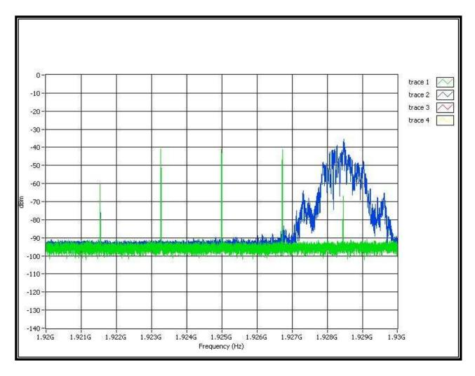
Note 1: The interference of level on f1 is TL+UM+1dB. The interference of level on f2 is TL+UM-6dB. The level of other 3 carriers is TU+UM.
