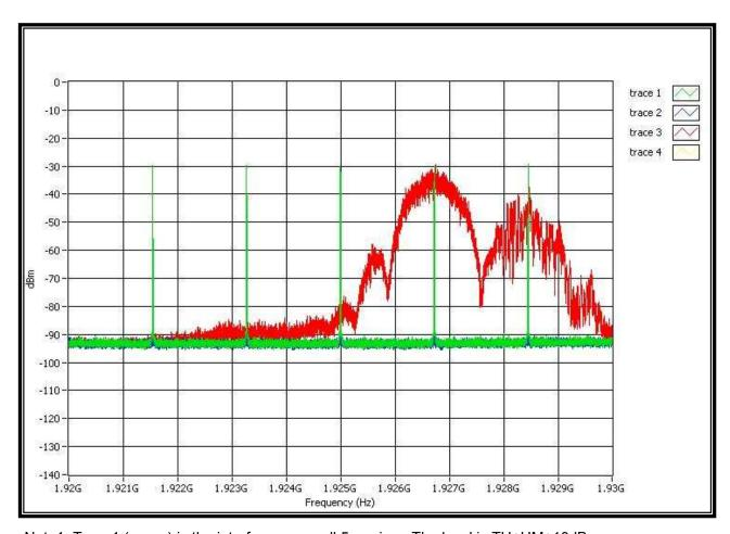
Note1: Trace1 (green) is the interference on all 5 carriers. The level is TU+UM+10dB.
