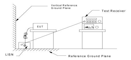
Test Set-Up 4
