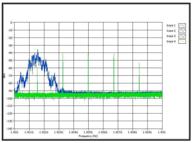
Note 1: The interference of level on f2 is TL+UM+7dB. The interference of level on f1 is TL+UM. The level of other 3 carriers is TU+UM.
