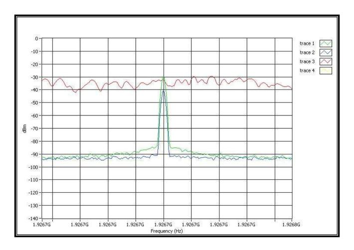
Note 1: Trace1 (green) is the interference on the carrier. The level is TU+UM+10dB.
