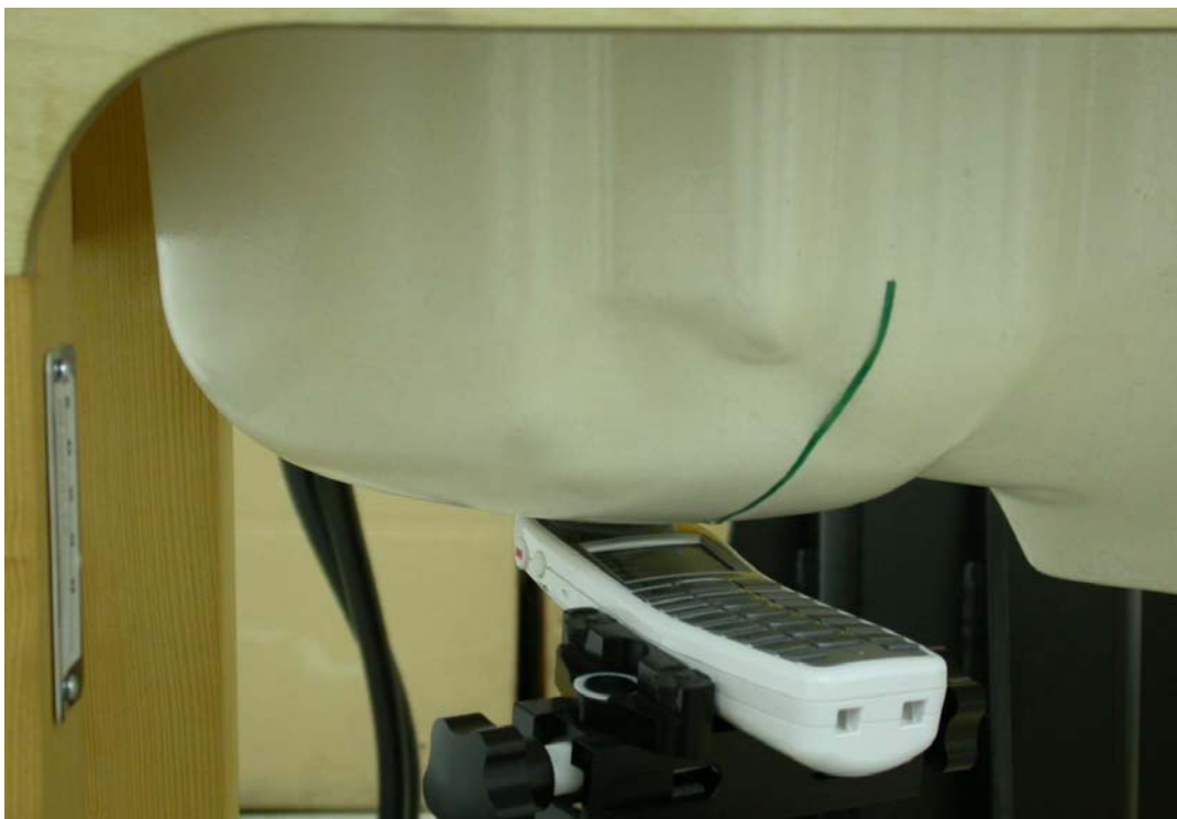
Measurement Position of Right-Tilt (RT) with Handset
