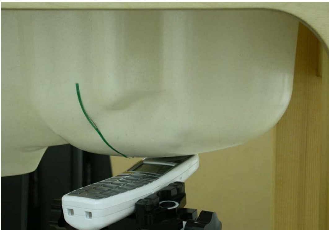
Measurement Position of Left-Tilt (LT) with Handset
