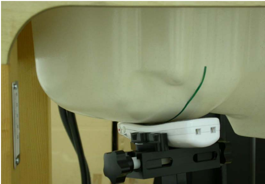
Measurement Position of Right-Cheek (RC) with Handset
