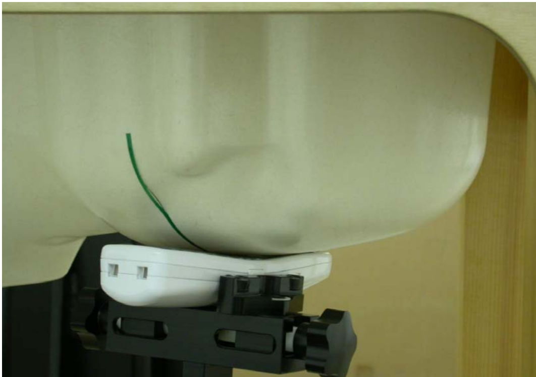
Measurement Position of Left-Cheek (LC) with Handset
