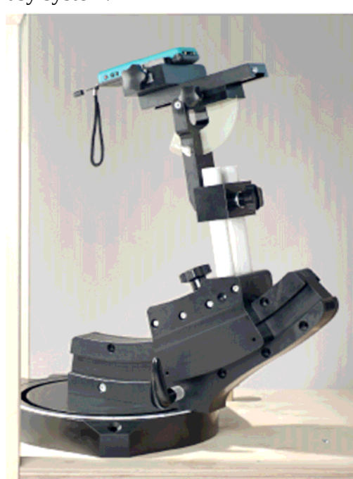
Fig. 10 Device holder supplied by SPEAG
