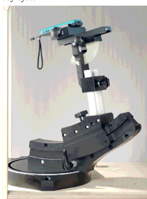
Fig. 10 Device holder supplied by SPEAG
