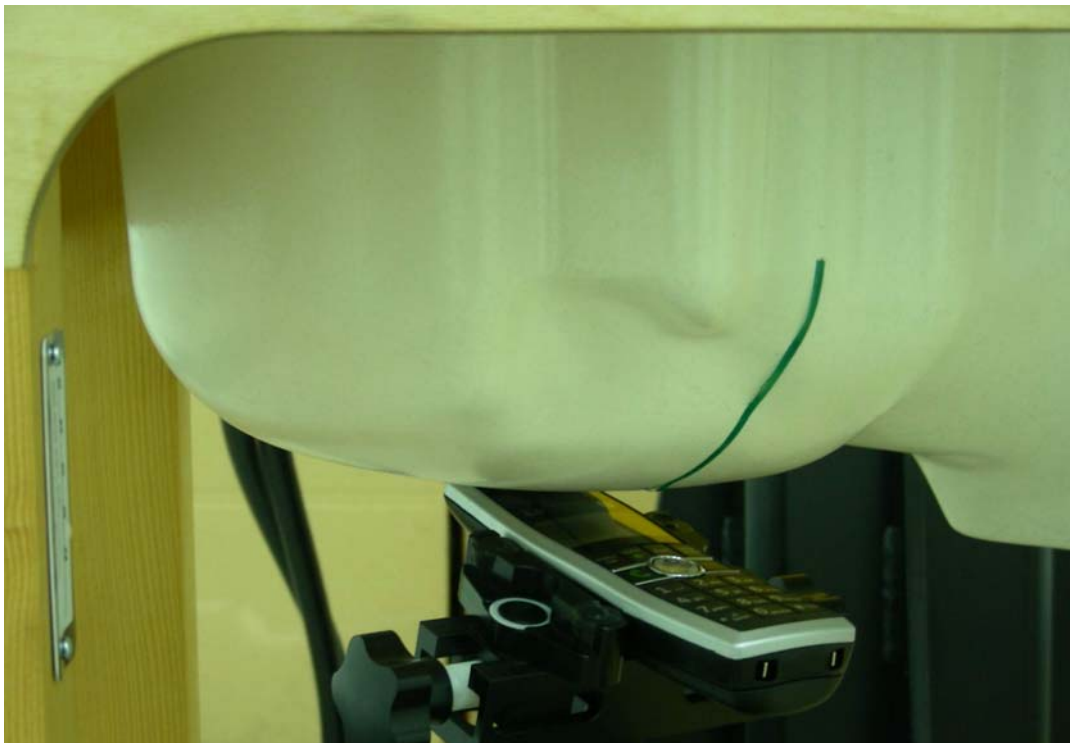
Measurement Position of Right-Tilt (RT) with Handset
