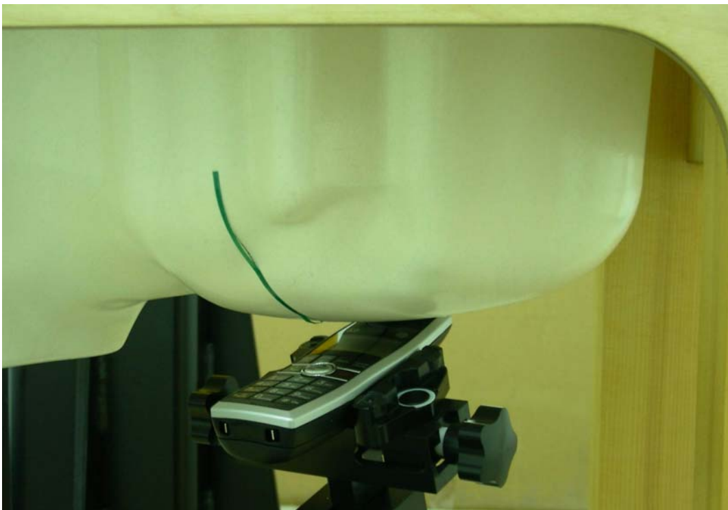
Measurement Position of Left-Tilt (LT) with Handset
