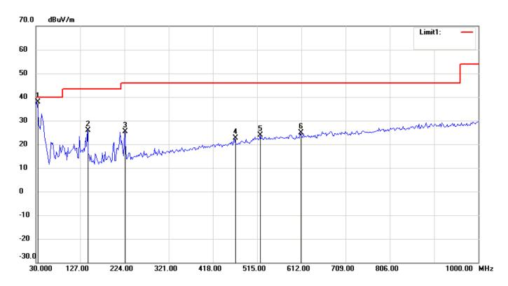
Condition: FCC Part15 RE-Class B\_30-1000MHz Polarization: Vertical
