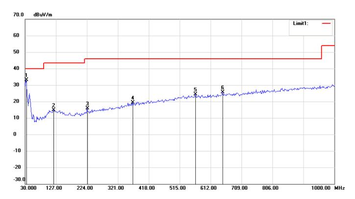
FCC Part15 RE-Class B\_30-1000MHz Condition: Polarization: Horizontal
