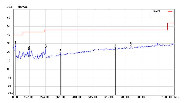
Condition: FCC Part15 RE-Class B\_30-1000MHz Polarization: **Vertical**
