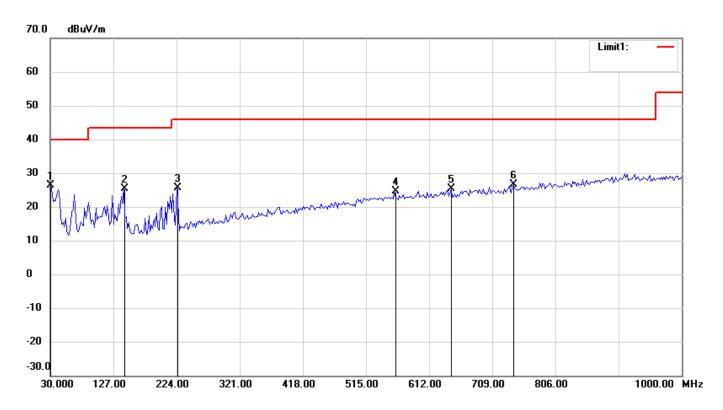
Condition: FCC Part15 RE-Class B\_30-1000MHz Polarization: Vertical
