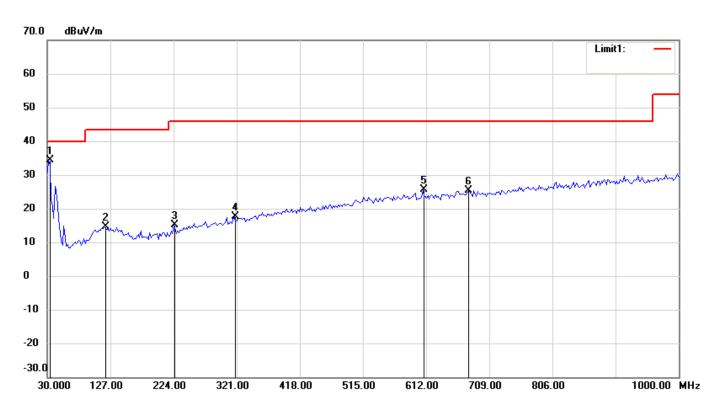
Condition: FCC Part15 RE-Class B\_30-1000MHz Polarization: Horizontal
