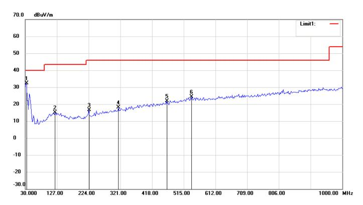
**Condition:** FCC Part15 RE-Class B\_30-1000MHz Polarization: Horizontal
