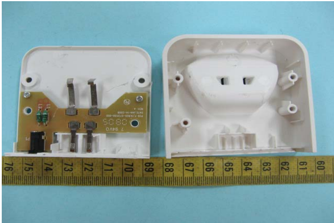
Internal View of Charger
