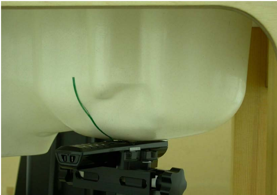
Measurement Position of Left-Cheek (LC) with Handset
