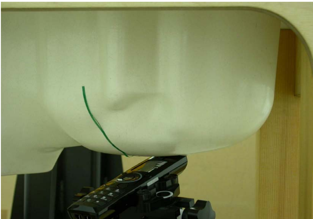
Measurement Position of Left-Tilt (LT) with Handset
