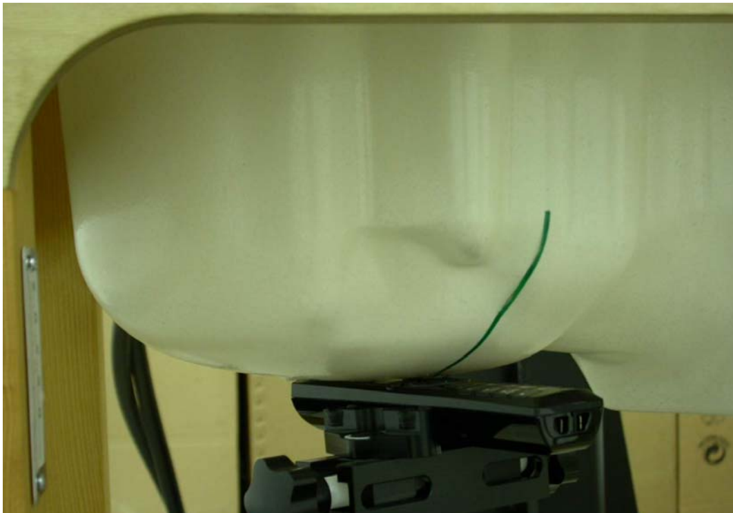
Measurement Position of Right-Cheek (RC) with Handset
