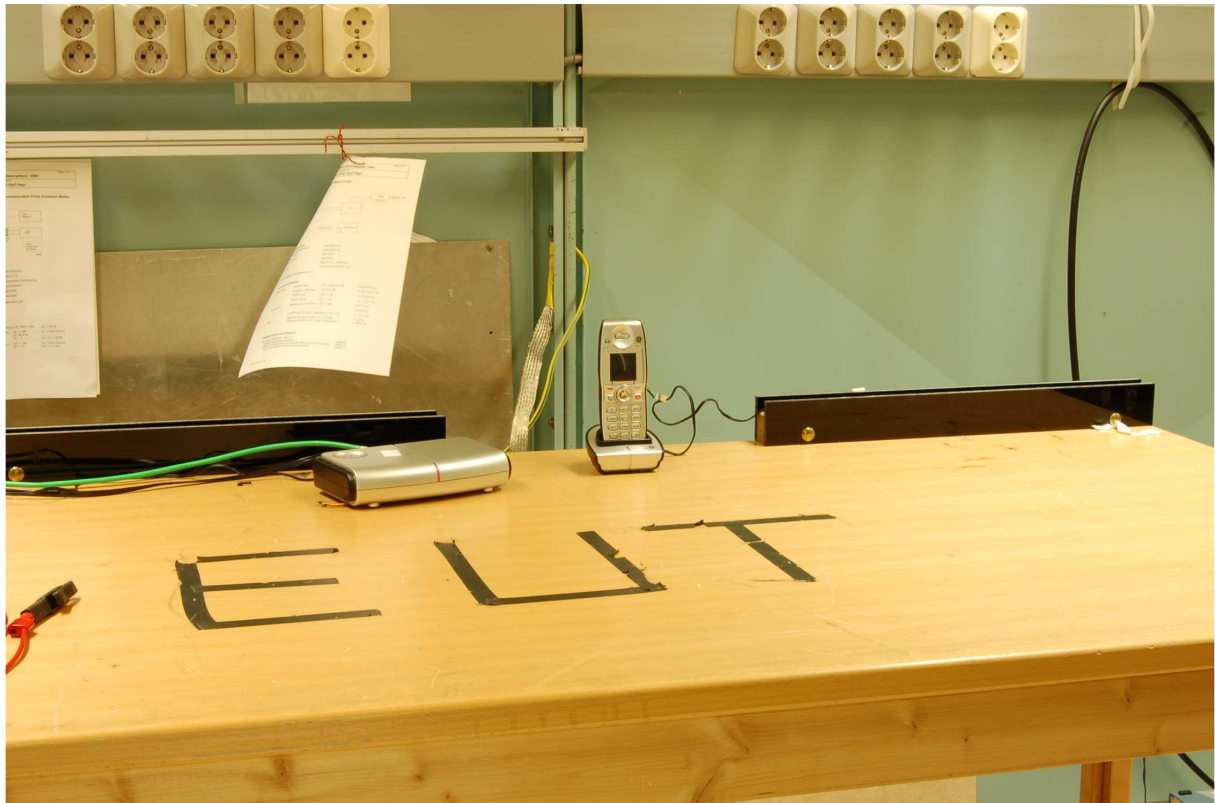
Power line Conducted Emissions Test
