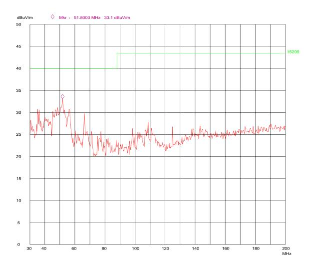
Spurious Emissions 30 – 200 MHz, Peak Detector, Vertical Polarization
