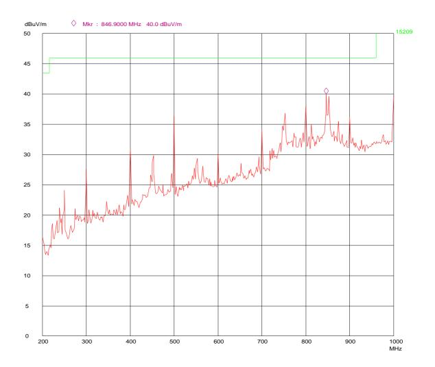
Spurious Emissions 200 - 1000 MHz, Peak Detector, Horizontal Polarization
