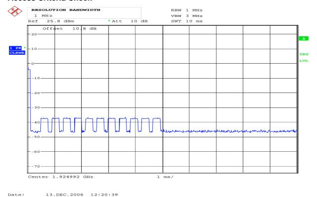
8.1.1a) EUT Transmits on Unblocked Slot
