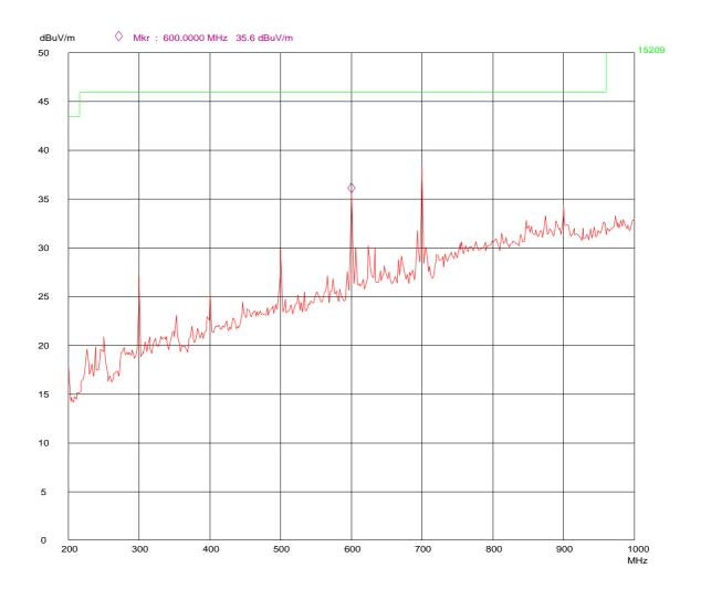
Spurious Emissions 200 - 1000 MHz, Peak Detector, Vertical Polarization
