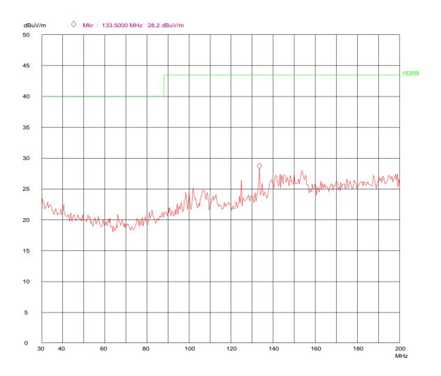
Spurious Emissions 30 – 200 MHz, Peak Detector, Horizontal Polarization
