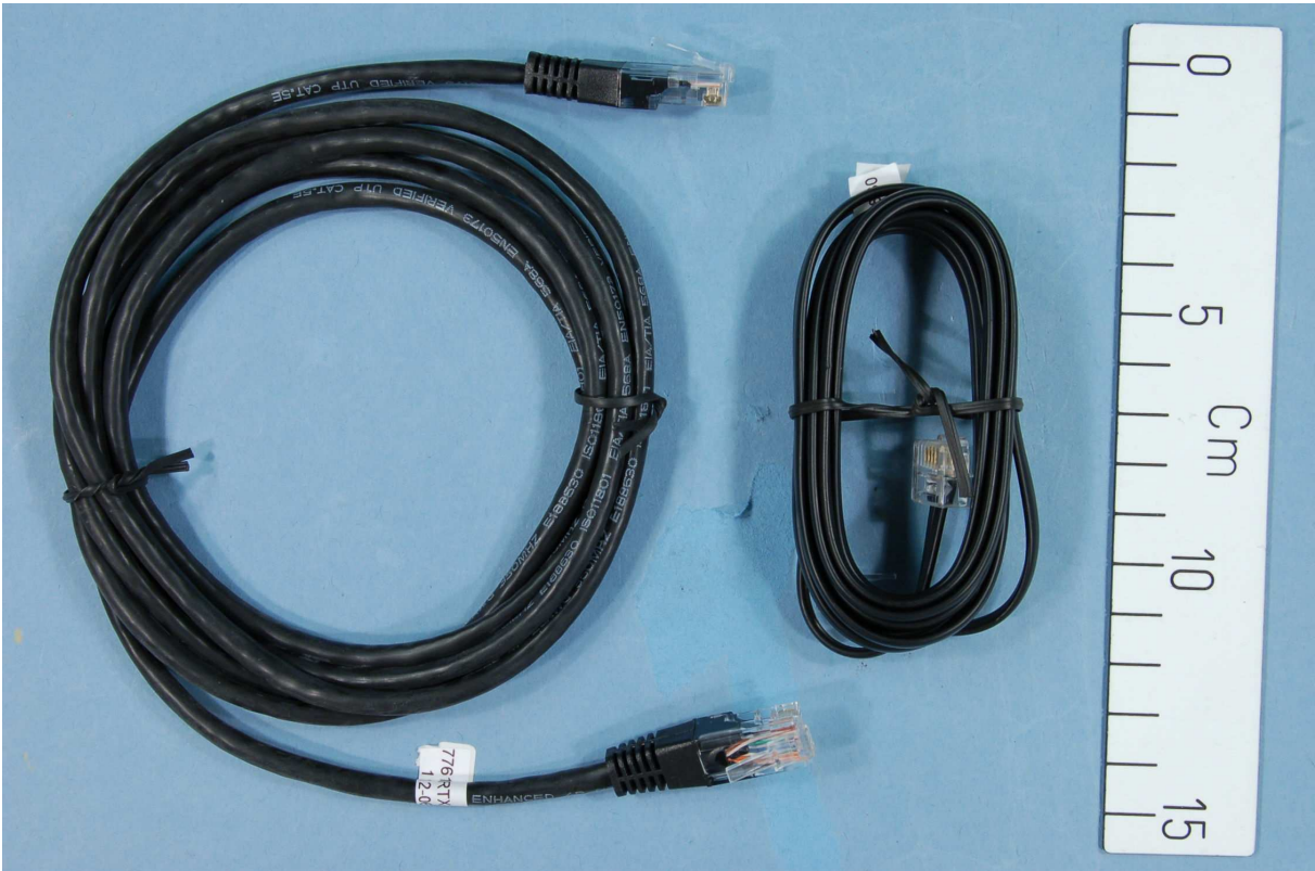
Tele Line and Ethernet Cables
