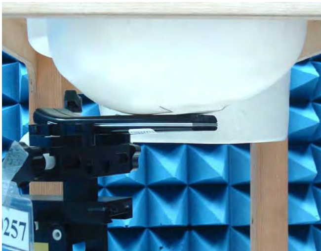
Figure 16. Left Head SAR Test Setup (Cheek)
