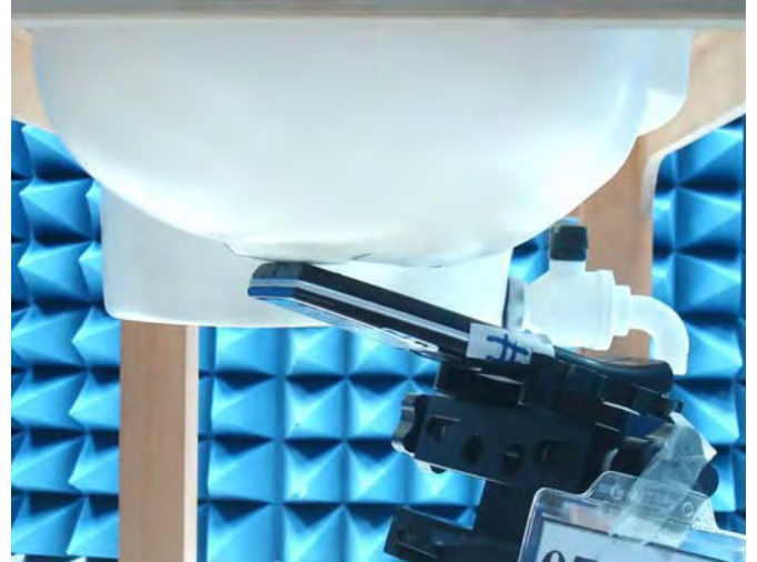
Figure 15. Right Head SAR Test Setup (Tilted)
