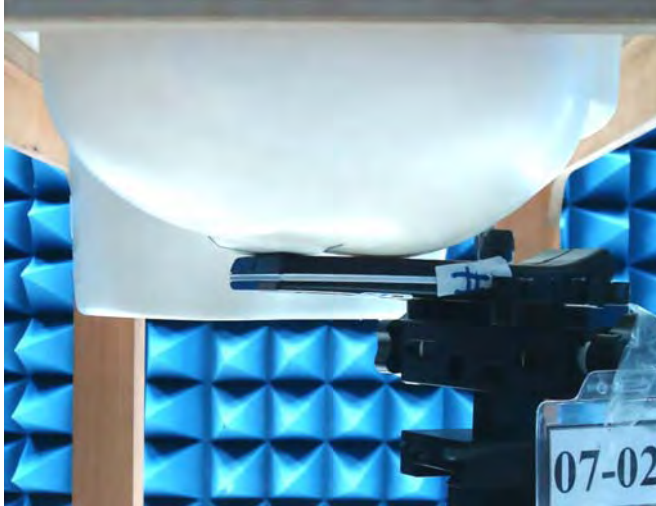
Figure 14. Right Head SAR Test Setup (Cheek)
