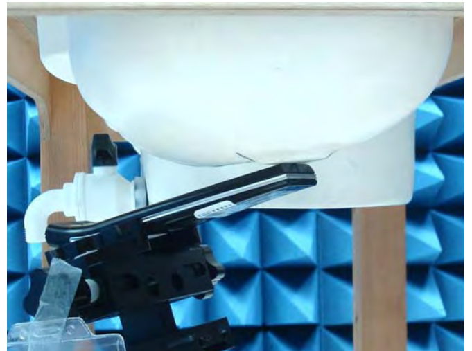
Figure 17. Left Head SAR Test Setup (Tilted)
