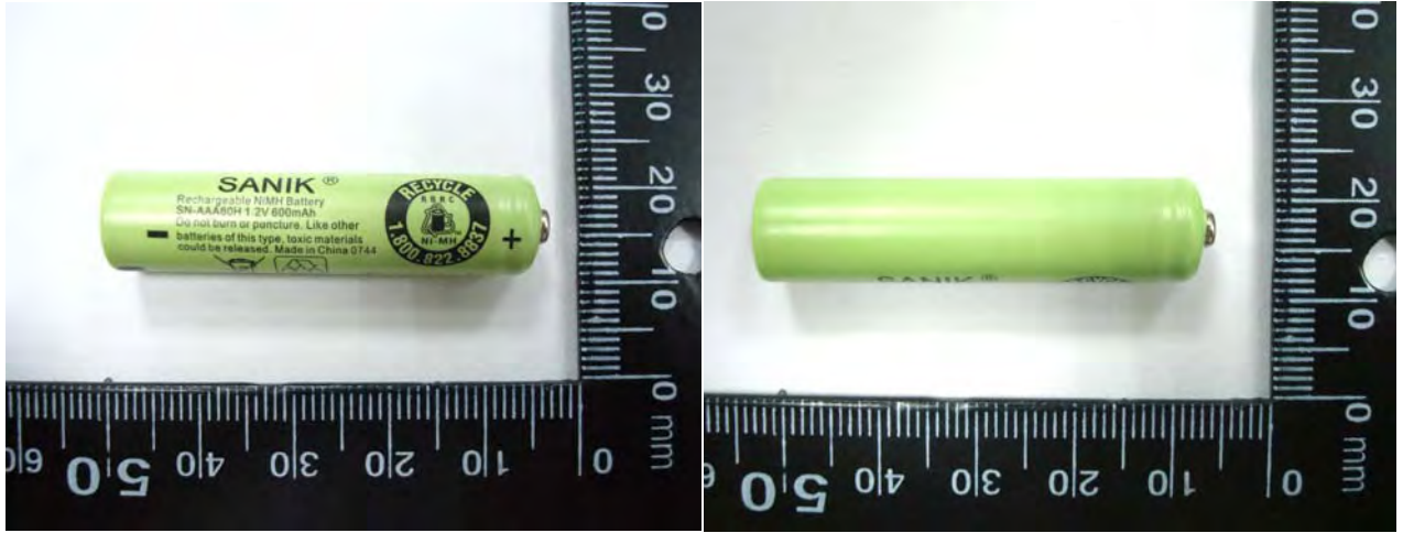
Figure 2. Battery (Ni-MH 1.2V , 600mAh)
