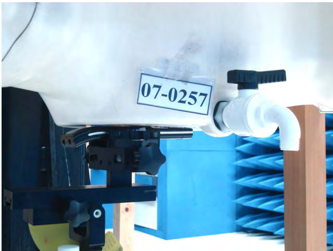
Figure 18. Body SAR Test Setup (Flat Section)
