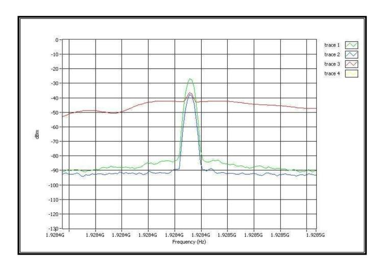
Note1: Trace1 (green) is the interference on all 5 carriers. The level is T∪+Uм+10dB.
