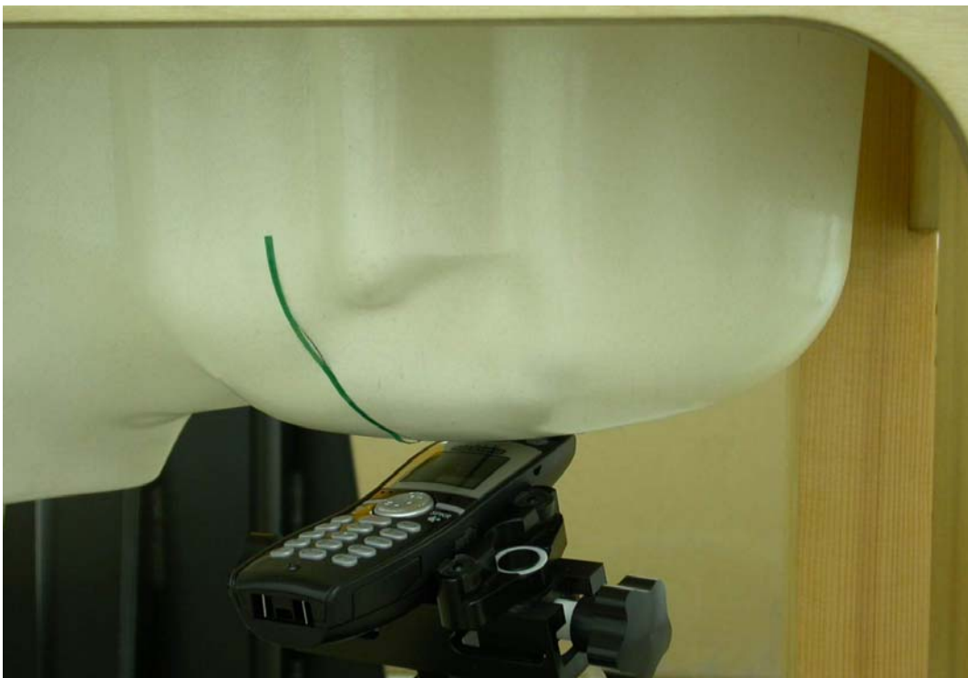
Measurement Position of Left-Tilt (LT) with Handset
