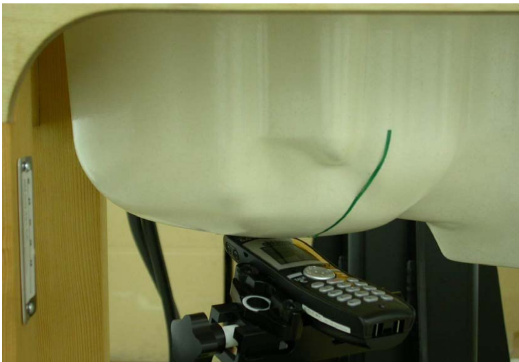
Measurement Position of Right-Tilt (RT) with Handset
