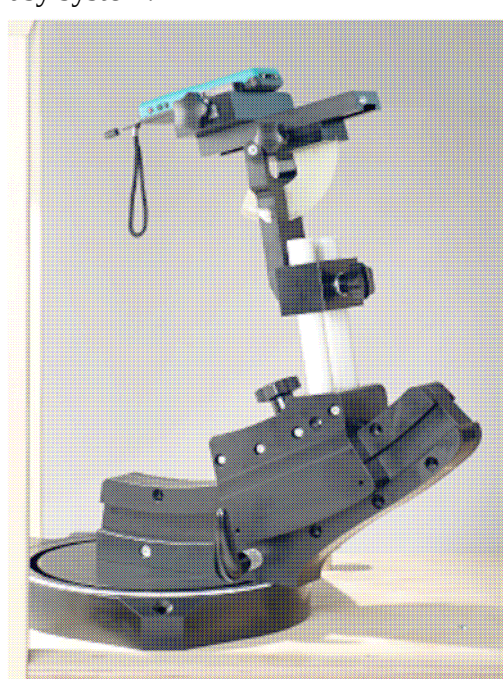
Fig. 10 Device holder supplied by SPEAG
