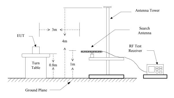
Figure 1: Frequencies measured below 1 GHz configuration
