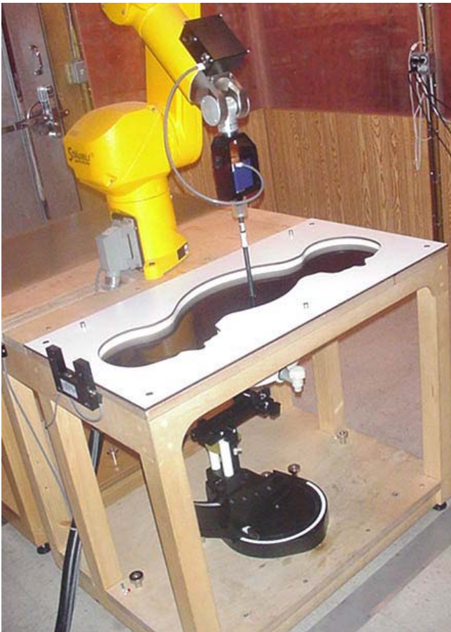
DASY4 SAR Measurement System with SAM phantom and 5GHz Fluid Left View
