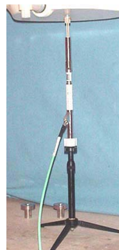
D5GHzV2 Dipole Setup
