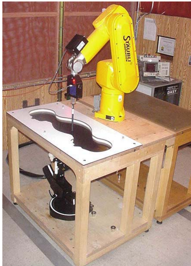
DASY4 Measurement System with SAM Phantom and 5GHz Fluid Right View
