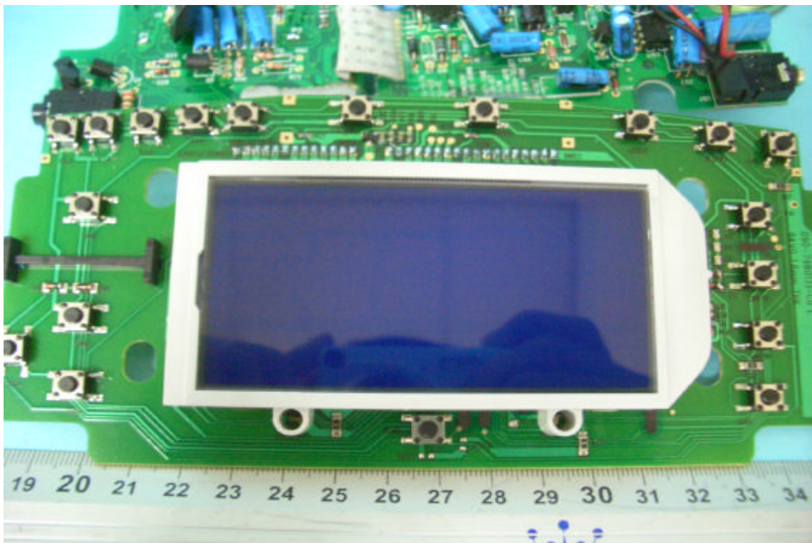
Solder View of Base Unit's Main PCB
