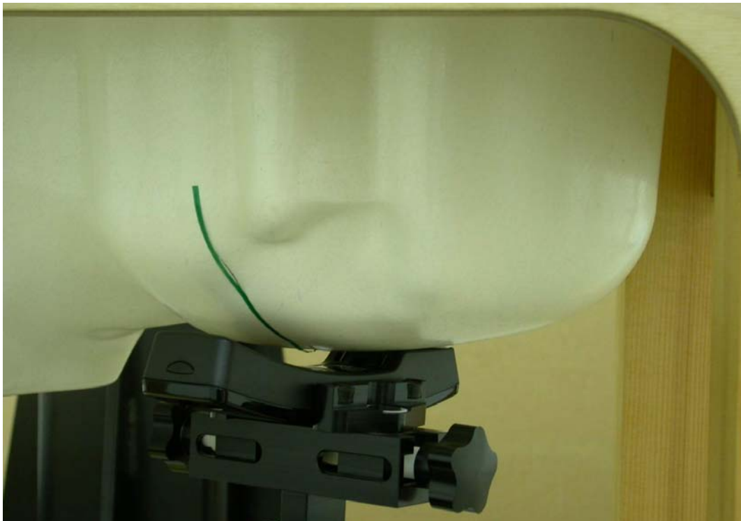
Measurement Position of Left-Cheek (LC) with Handset
