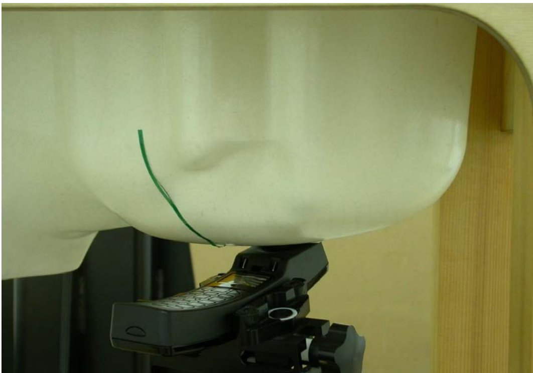
Measurement Position of Left-Tilt (LT) with Handset
