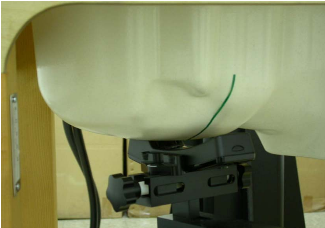
Measurement Position of Right-Cheek (RC) with Handset
