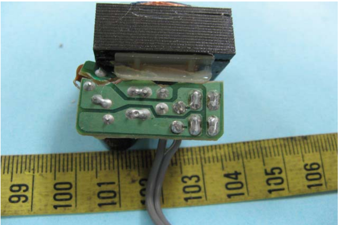
Solder View of Adaptor's PCB
