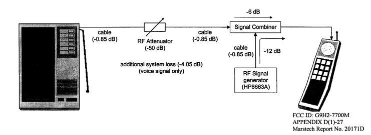
The following parameters were used in the test setup.
