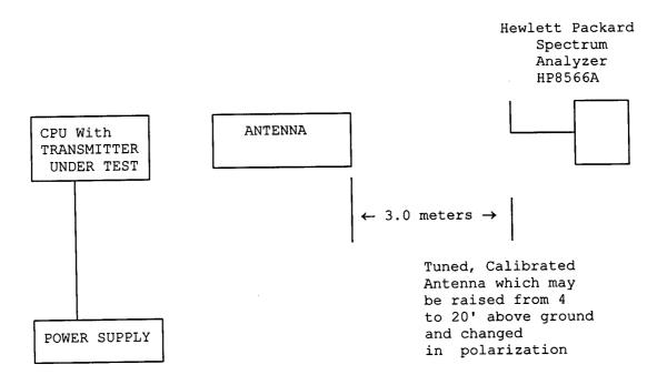
Equipment placed 4' above ground on a rotating platform.
