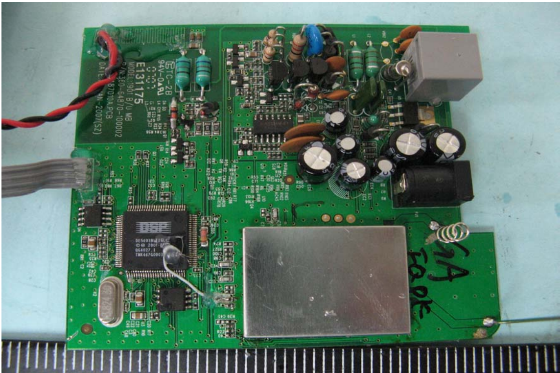
Component View of Base Unit’s Main PCB
