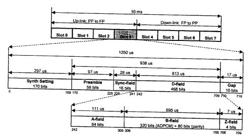
The basic, repeating, frame structure is 10 ms long. It is sub-divided into 8 slots, each 1250  $\mu$ s long. The active transmission time is 937.5  $\mu$ s. The first 4 slots form the 'up-link', when the PPs transmit to the FP. The last 4 slots form the 'down-link', when the FP transmits to the PPs.
