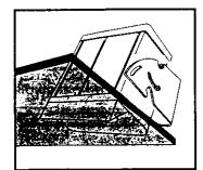
The sensor must not be placed behind a panel or any kind of material
