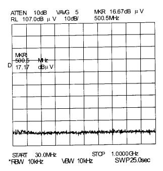
No measurable signal have been detected higher than the noise level which, with the GTEM conversion chart is far lower than the acceptable limits.
