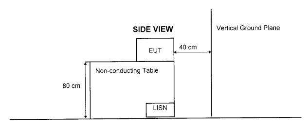
Other Measurements: 2 meters from top of EUT to ceiling 80 cm from closest part of EUT to the LISN
