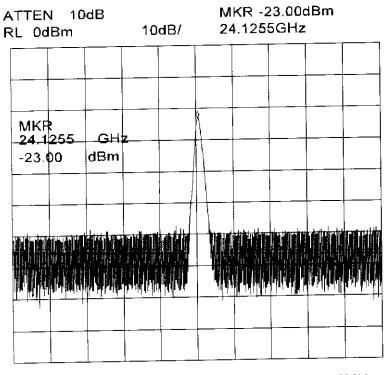
CENTER 24.1250GHz SPAN 100.0MHz RBW 1.0MHz VBW 1.0MHz SWP 50.0ms
