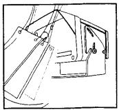
No object which could move or vibrate must be present within the sensing field
