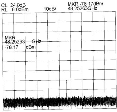
CENTER 48.25200GHz \*RBW 3.0kHz VBW 3.0kHz SPAN 10.00MHz SWP 2.80sec
