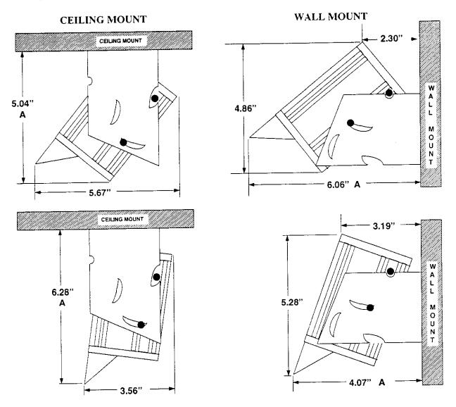
3. Use the mounting bracket as a template to locate holes on surface of mounting location. Dimensions are shown below. DO NOT exceed a mounting height of 20.0'. Excessive height may cause erratic detection of traffic.
