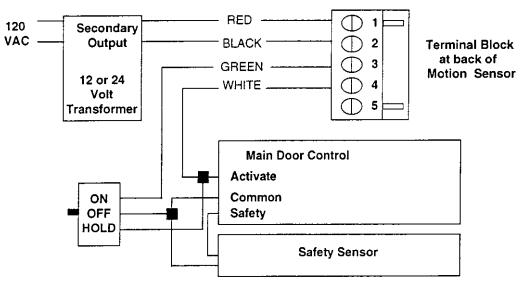
\*Wiring shown is for a door control requiring normally open contacts for activation. If normally closed is required, use terminals 3 & 5 on motion sensor terminal block.
