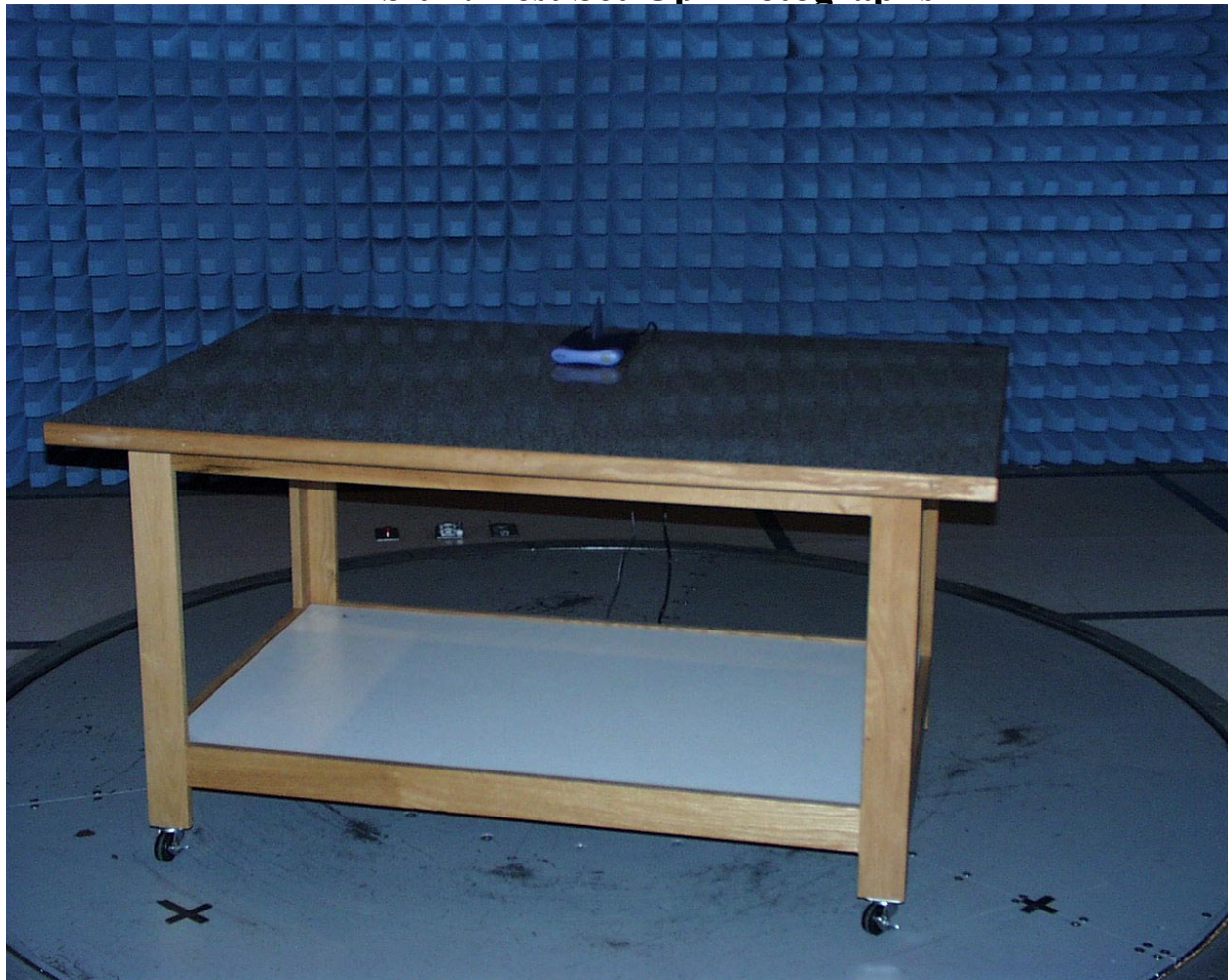
Front View of Worst Case Radiated and Line Conducted Emissions Test Set-up
