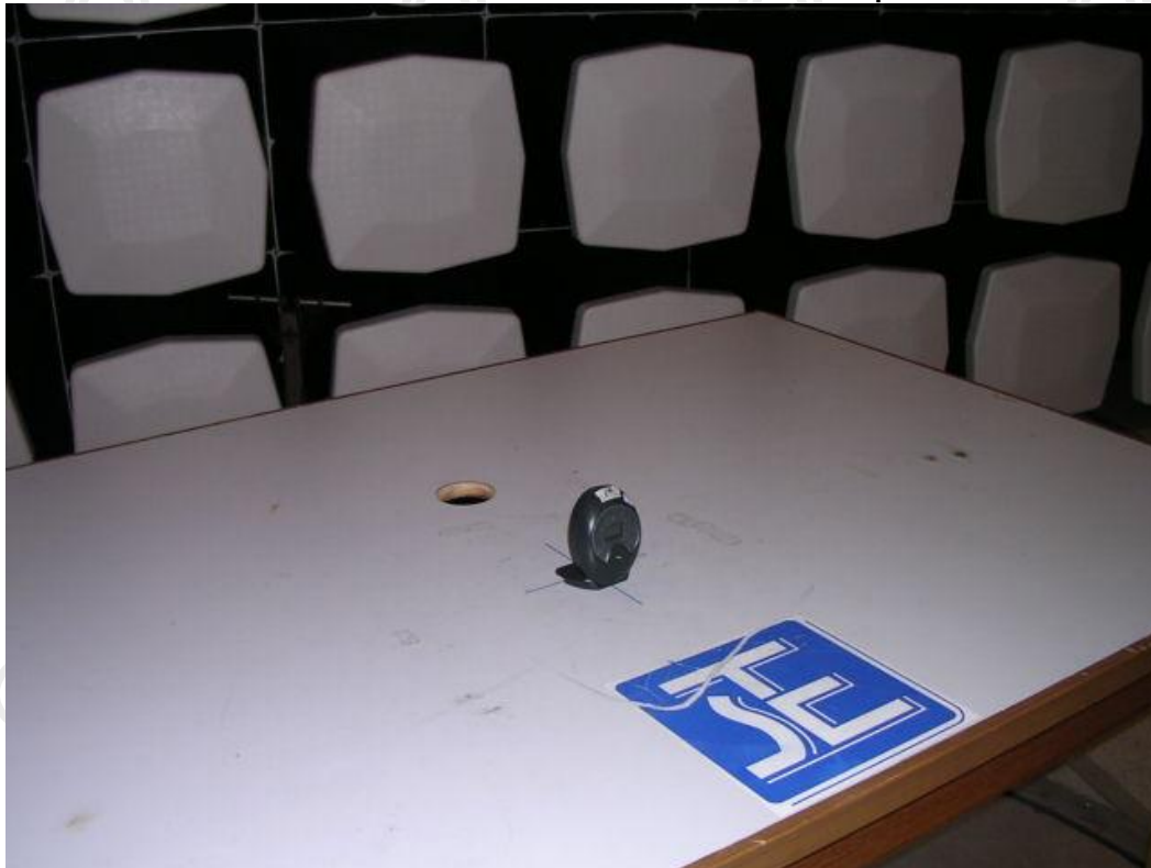
Measurement of Radiated Emission Test Set Up
