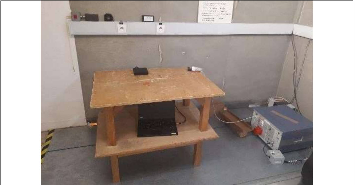
Photograph for AC Power Line Conducted Emissions (Front view)
