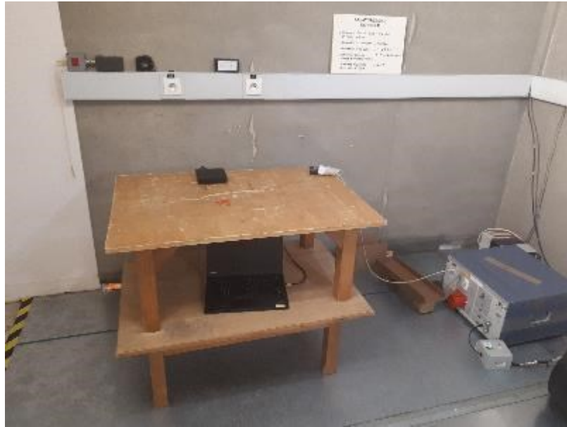
Photograph for AC Power Line Conducted Emissions (Front view)
