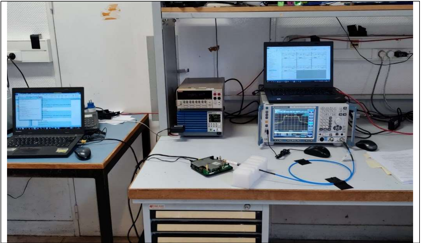
Photograph for Occupied bandwidth
