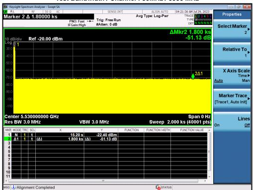
Test Bandwidth / Channel: 80MHz / 5530 MHz
