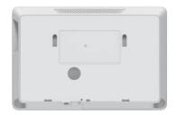
2. Remove the back plate from the back of the touchscreen by pulling the center of the bottom edge upward, then sliding the top tabs out of the slots.
