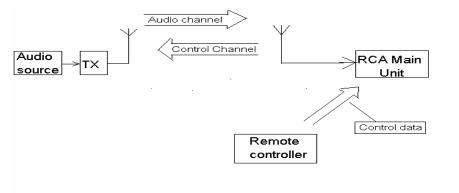
The MAIN UNIT(MU), USB DUNGLE(UD) and REMOTE CONTROLLER(RC) are a complete system. The system is based on wireless digital audio transfer from an audio source to MAIN UNIT, and REMOTE CONTROLLER can control MAIN UNIT by radio. It is noted that the communication between USB DUNGLE and MAIN UNIT are based on half-duplex transmission, MAIN UNIT and REMOTE CONTROLLER are base on simplex transmission.
