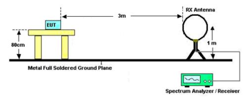
For radiated emissions from 30MHz to 1GHz <CDD Mode>
