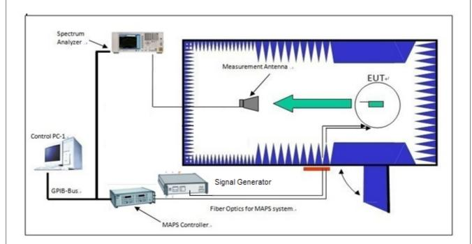
Figure 1. 2D antenna pattern test system.
