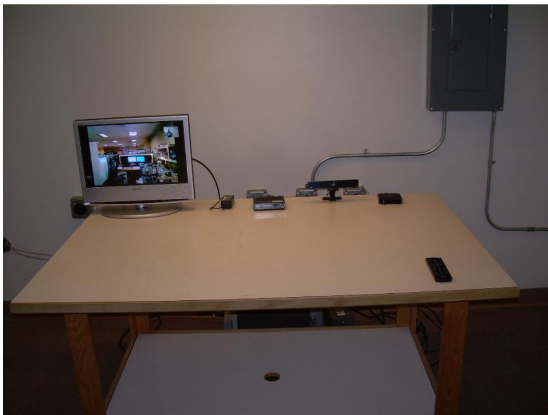
Front View Conducted Disturbance Test Configuration
