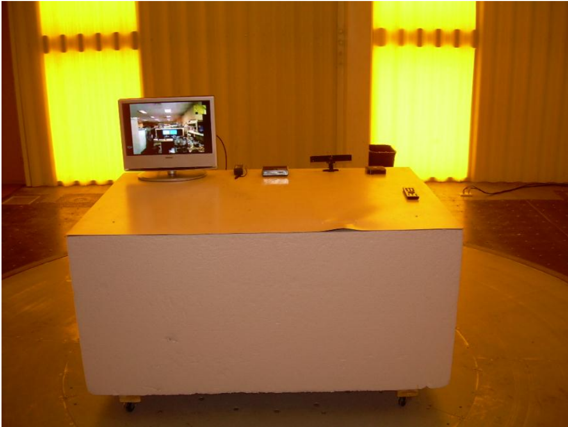
Front View Radiated Disturbance Test Configuration
