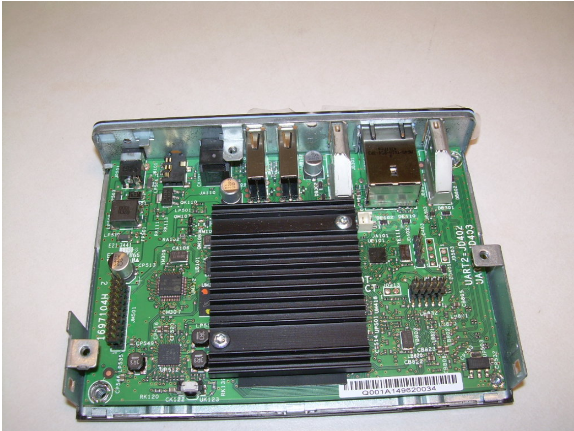
Photograph 10 – Top View of the Main PCB with Heatsink in Place
