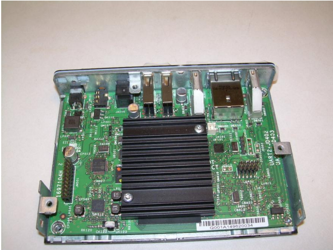
Top View of the Main PCB with Heatsink in Place
