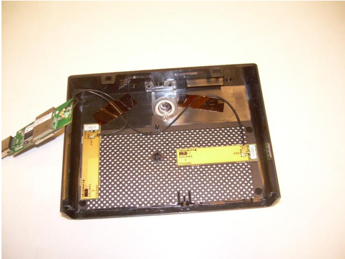
View of the Top Housing with the 802.11abgn Module and Antennas
