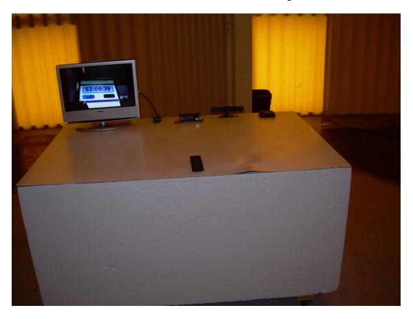
Back View Radiated Disturbance Test Configuration
