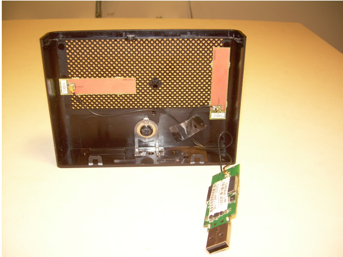
Photograph 18 – View of the Top Housing with the 802.11abgn Module and Antennas
