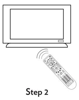
Install the batteries (*included in your kit*) in your new remote control. Press and hold both Digit 1 and Digit 3 buttons together until the red light turns on. Release both buttons.
