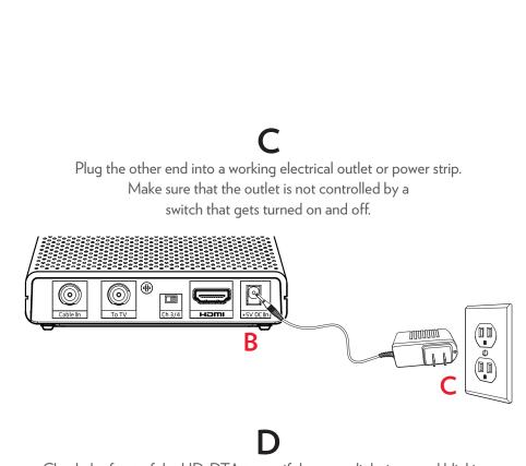
Check the front of the HD-DTA to see if the green light is on and blinking. If it is not on, check to make sure the power plug was plugged into the power input "+5V DC In" and that the other end is plugged into a working electrical outlet.
