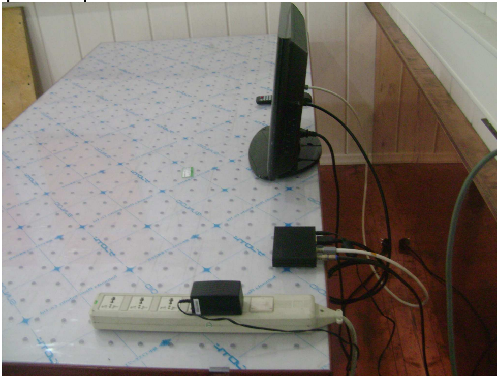
Photograph 2: Set-up for Spurious Emissions 30MHz – 1GHz
