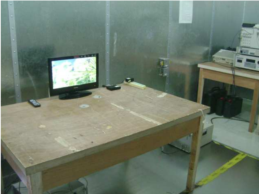
Photograph 2: Set-up for Spurious Emissions 30MHz – 1GHz
