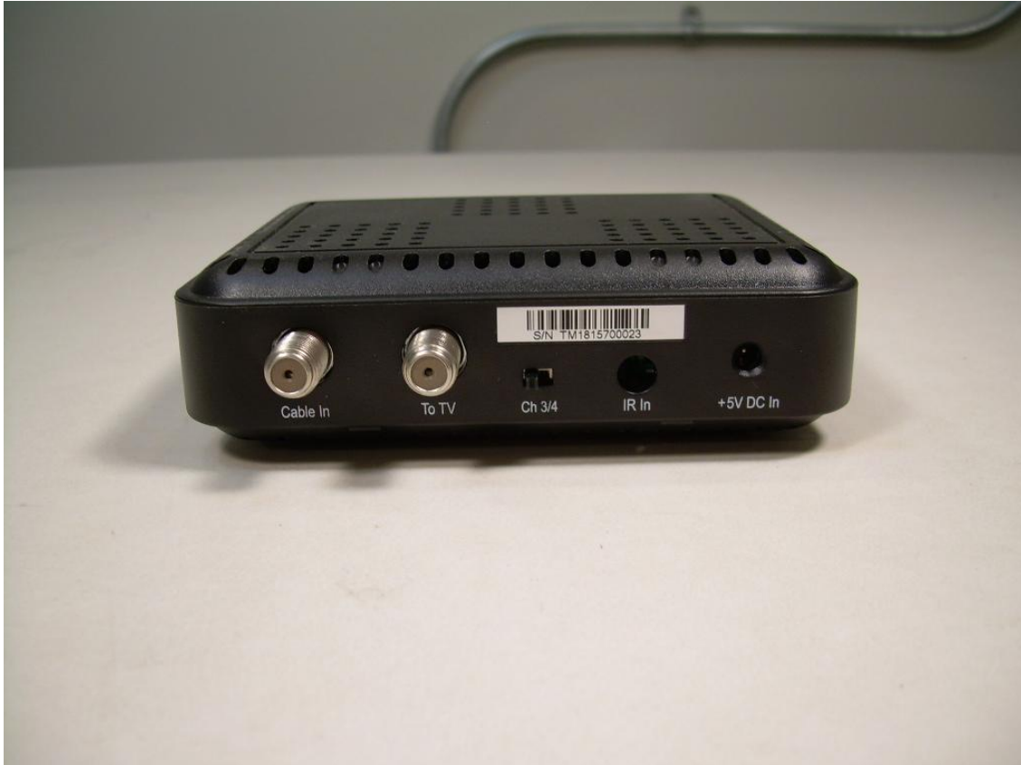
Photograph 6 – Back View of the DCI104XXX Chassis
