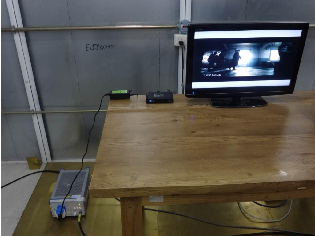
Photograph 2: Set-up for Radiated Emissions, below 1GHz
