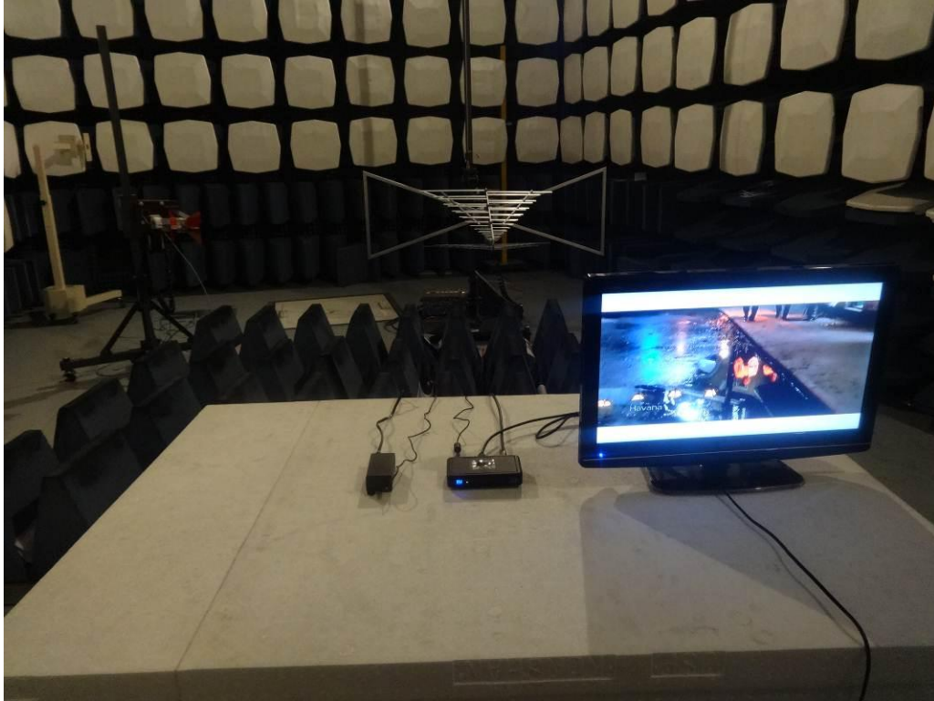
Photograph 3: Set-up for Radiated Emissions, above 1GHz
