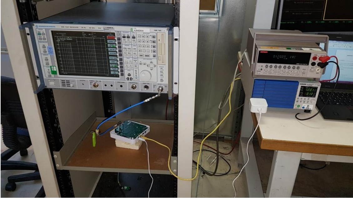
Photograph for Unwanted Emission into non-restricted frequency bands (BT Classic)
