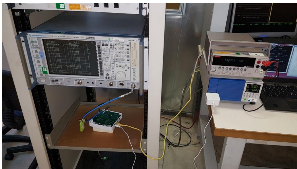
Photograph for Unwanted Emission into non-restricted frequency bands (Wifi 2.4GHz)
