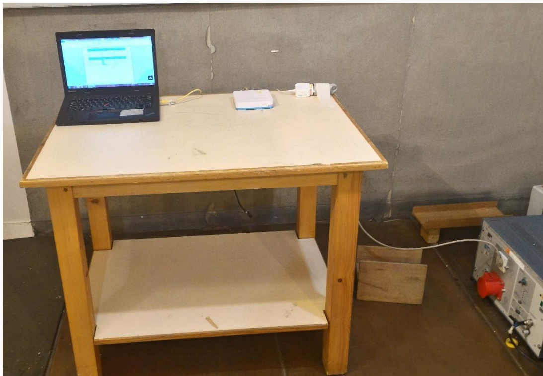
Conducted emission measurement setup
