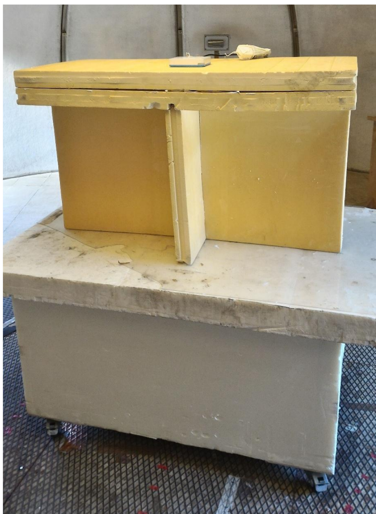
Radiated emissions measurements setup above 1GHz
