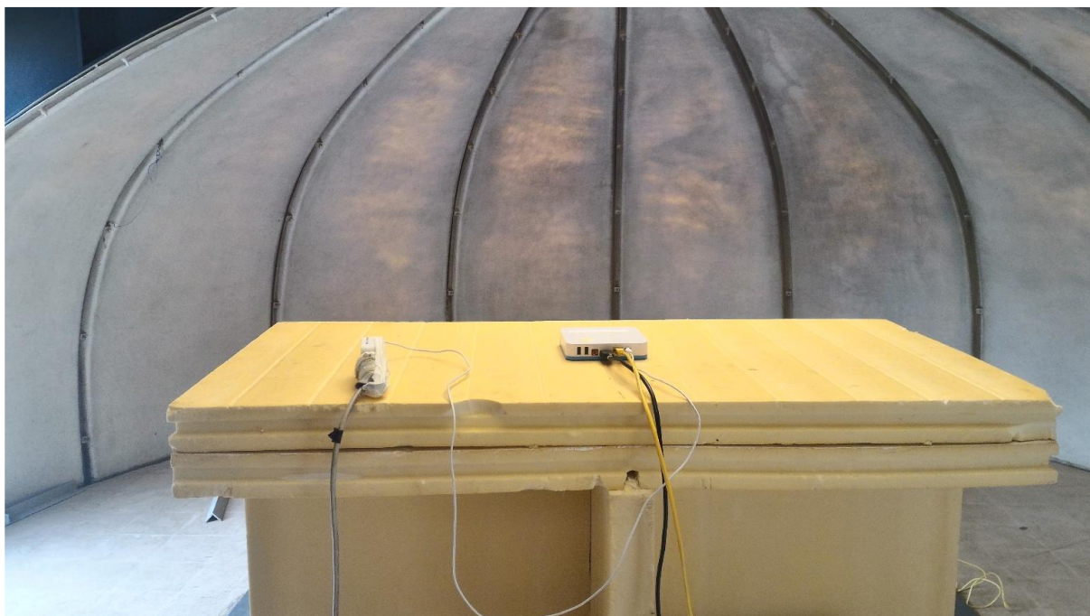
Radiated emissions measurements setup above 1GHz
