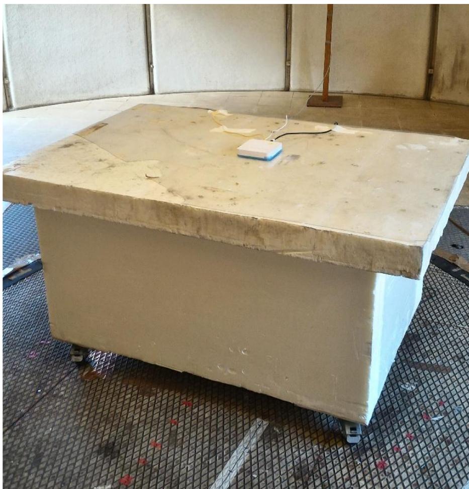
Radiated emissions measurements setup below 1GHz
