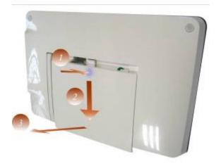
2. Connect the battery connector and insert the battery in its compartment.
