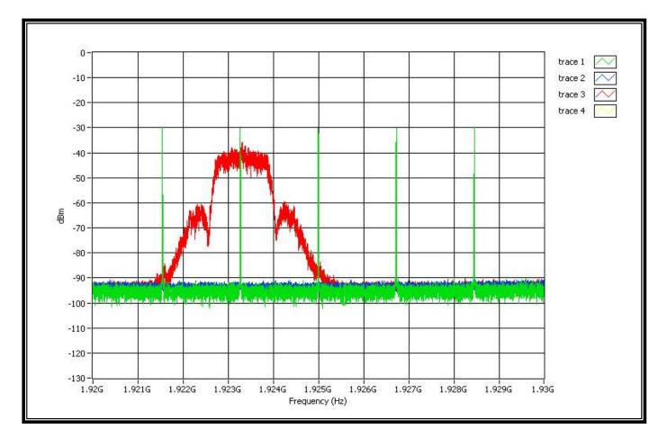
Comment1: Trace1 (green) is the interference on all 5 carriers. The level is Tu+UM+10dB. Comment2: Trace2 (blue) is interference on all 5 carriers. The level is TuR. Comment3: Trace3 (Red) is the EUT begins to transmit the beacon when interference is TuR. Comment: 7.3.2 (zoom in)
