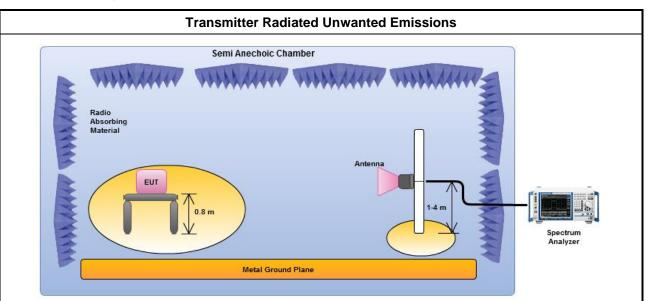
Magnetic field tests shall be performed in the frequency range of 9 kHz to 30 MHz using a calibrated loop antenna. Electric field tests shall be performed in the frequency range of 30 MHz to 1000 MHz using a calibrated bi-log antenna and the frequency range of 1 GHz to 40 GHz using a calibrated horn antenna.
