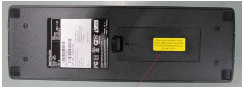
Battery label Position 貼于label框內
