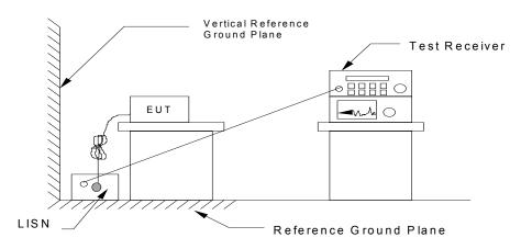
**Test Set-Up 4**
